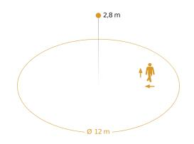
Possible mounting height: 2,50 m – 4,00 m Orange: radial and tangential
